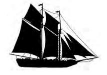
A slender, swift shallow-draft ship with two masts rigged fore-and-aft.
