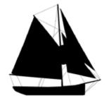
A small, fast, rakish vessel with a single fore-and-aft rigged mast; favored by freebooters and smugglers, but also used as local guard ships (hired by coastal towns to battle pirates). The best were "Bermuda sloops" built out of red cedar.
